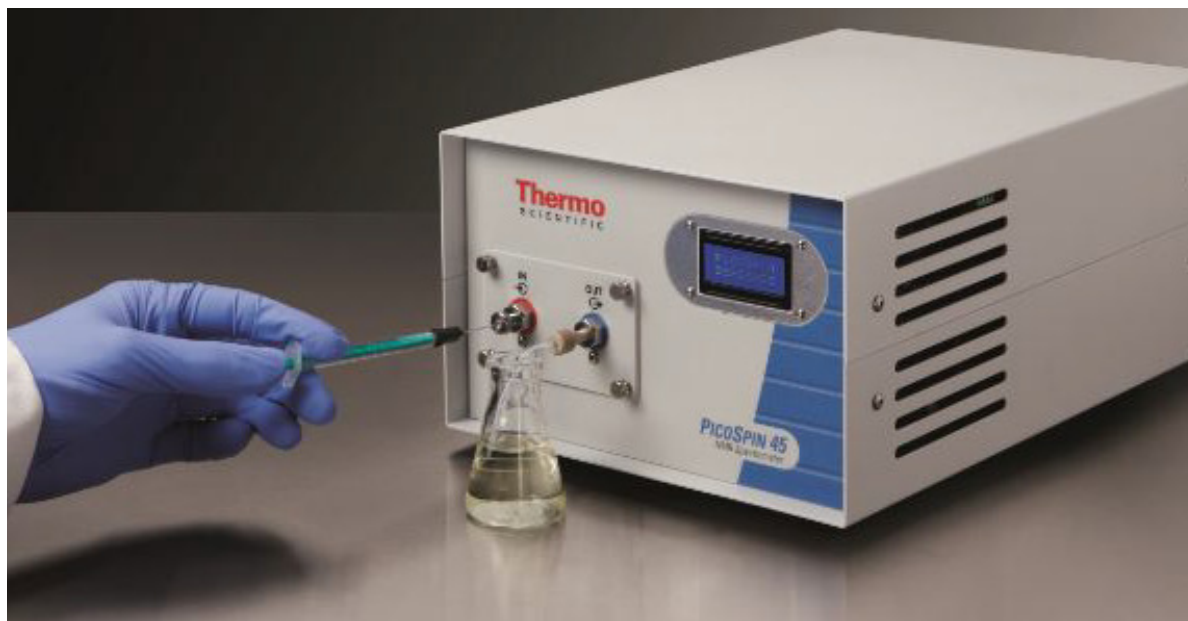
Figure 3. Fill and drain tubes attached and ready for injection
